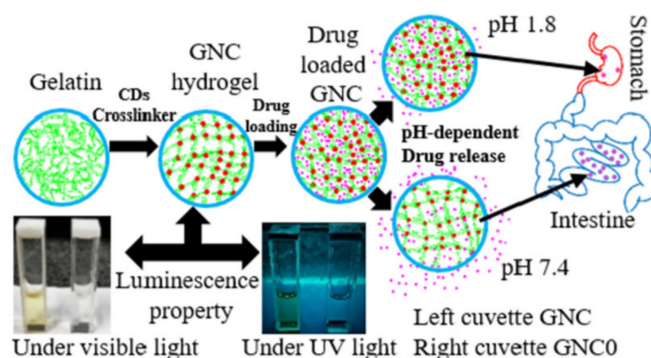
Figure 5. Formation of the gelatin nanocomposite crosslinked with carbon dots and loaded with a drug that is released in the gastrointestinal tract. The gelatin nanocomposite (GNC) hydrogels show fluorescence properties for biosensing and measuring the pH of the digestive system. Reprinted with permission from reference [88]. Copyright 2020 American Chemical Society.
