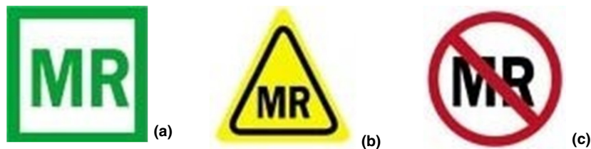
Figure 2. Icons used in the ASTM F2503-20 standard for MR safety category labelling: (A) MR Safe, items that pose no known risk or hazard in the MRI environment; (B) MR Conditional, implants and devices demonstrate no hazard in the MRI environment, but only when prescribed conditions for safe use are adhered to; (C) MR Unsafe, implants and devices should never be brought into the MRI environment. 21
