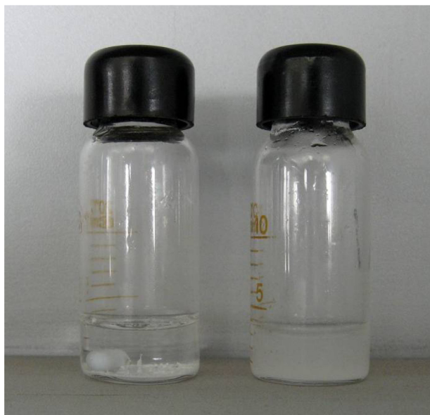
Figure 1 After stirring for 48 hours, paclitaxel 1 mg/mL in pure water was still clear (left). However, the same concentration of paclitaxel in 0.5% RADA16 aqueous solution was changed to a colloidal suspension (right).
