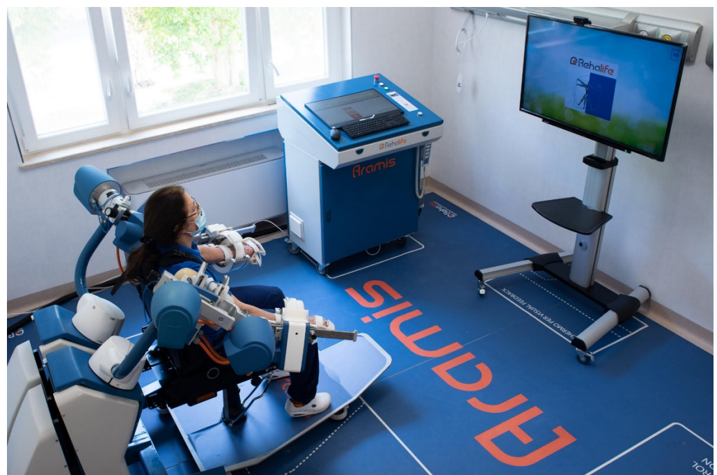
Figure 1. The robotic-assisted device called Automatic Recovery Arm Motility Integrated System (ARAMIS).
