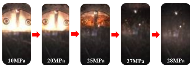
Figure 7. Miscible process of CO 2 and crude oil.
