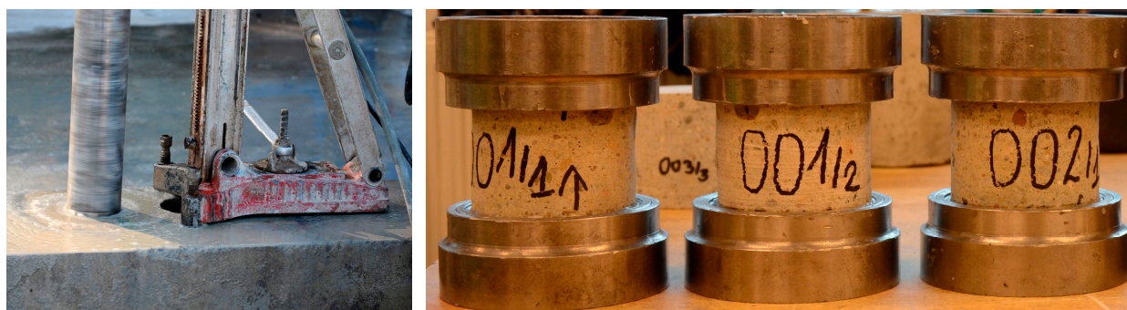
Figure 12. Testing for strength: core drilling and concrete specimens prepared for testing.
