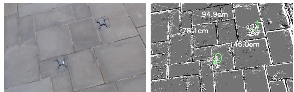
Figure 12. Experiments involving 2 quadrotors carried out in outdoor environments are depicted in RGB (left) and event (right) format. For the outdoor experiments, the RGB and event cameras were mounted at different locations on the imaging quadrotor. Due to the different camera perspectives, the quadrotors appear to be at slightly different positions in the RGB and event images shown here.
