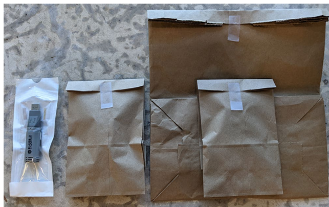
Figure 1. Sealed bags left to right: steam sterilization pouch, single layer paper bag, double layer (grocery and lunch size) paper bags.
