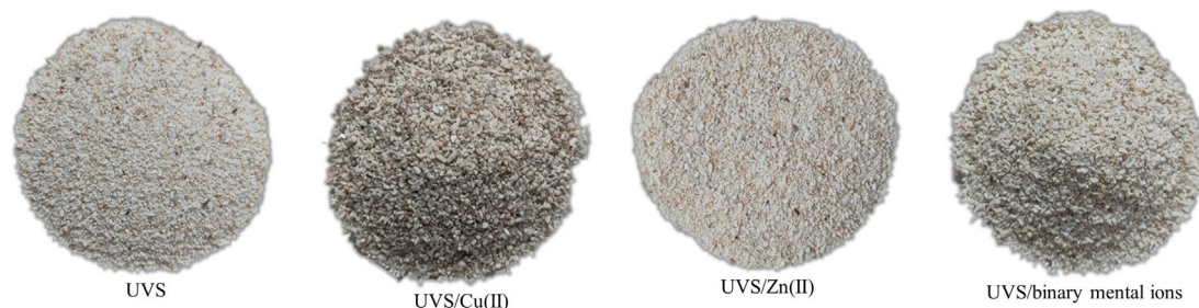
Figure 1. Untreated Venus shell (UVS) samples (from left to right): before adsorption, after adsorption with Cu(II), after adsorption with Zn(II), and after adsorption with binary Cu(II)/Zn(II).
