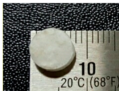
Figure 2. Photographs of PCL/PLGA/ \beta -TCP composite block bone grafts, 8 mm in diameter and 2 mm in height.
