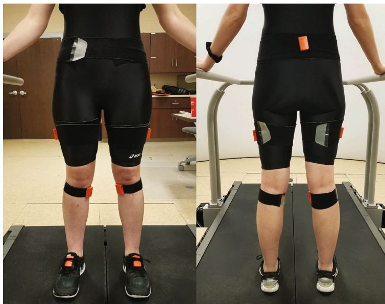
Fig. 5 IMU-based motion capture sensor (orange) setup for data collection
