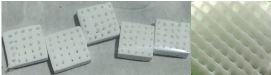
Figure 1: Three-dimensional printed \beta -TCP scaffold, 10×10×3 mm with 4-mm 2 channels.
