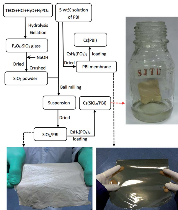
Fig. 1 Flow chart of the preparation of all the samples involved in this work. The photographs show pure PBI, an \text{SiO}_2/\text{PBI} matrix, and a \text{Cs}(\text{SiO}_2/\text{PBI}) electrolyte membrane.
