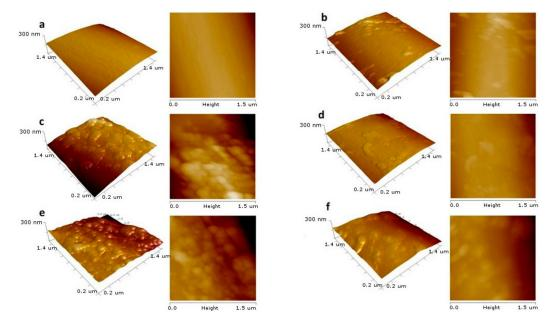
**Figure 3.** 2D and 3D height images of obtained surfaces from the AFM tapping-mode analysis, showing the influence of oxidation/unsheathing on the morphology of CNT layers created after the EPD process: (a) CF before the EPD, (b) oxidation time 10 min, (c) 15 min, (d) 30 min, (e) 75 min, (f) 90 min.
