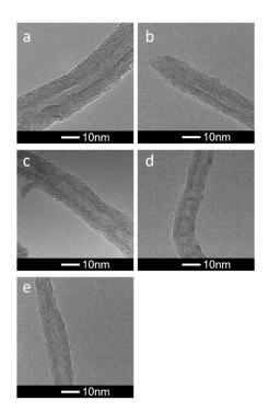
**Figure 1.** HRTEM images showing the influence of oxidation/unsheathing on the thickness of CNTs applied during the EPD process for oxidation times: (**a**) 10, (**b**) 15, (**c**) 30, (**d**) 75, (**e**) 90 min.
