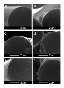
**Figure 2.** SEM images showing the influence of oxidation/unsheathing on the morphology of CNT layers formed after the EPD process: (a) CF before the EPD, (b) oxidation time 10 min, (c) 15 min, (d) 30 min, (e) 75 min, (f) 90 min.
