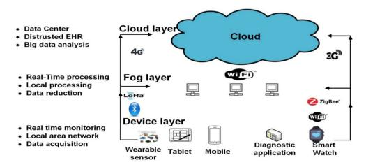
Figure 4. Fog computing layers in RPMs.
