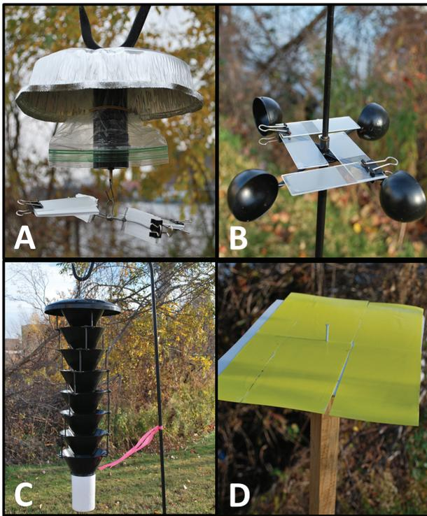
**Fig. 1.** Photos of each trap design used in this study: (A) motorized trap, (B) passive trap, (C) funnel trap, and (D) sticky trap.
