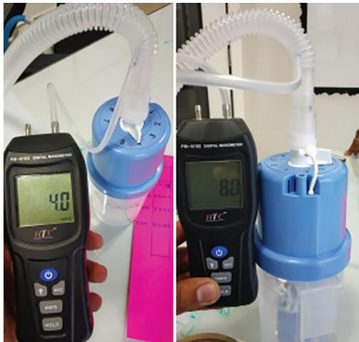
Annexure Fig. 1: Sampling pressure values in the circuit
