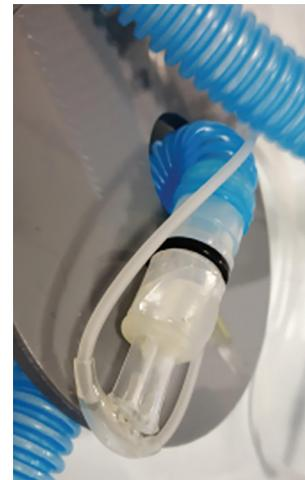
Annexure Fig. 2: Simulated nares, connects to test lung
