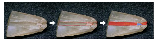
Figure 2. Methodology of residual materials area measurements using VHX-5000 software.
