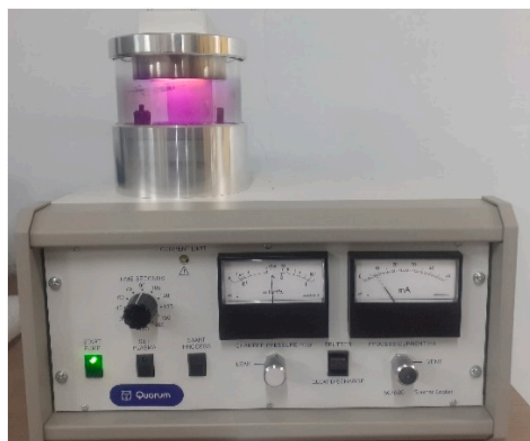
Fig. 4. Au-Pd (Gold-Palladium) plating on the SEM samples at CNSNT, ITER Laboratory.
