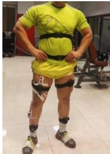
Figure 1. Noraxon’s myoMotion and myoMuscle sensor location.
