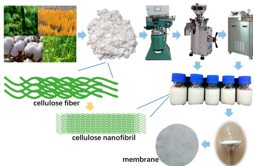
Figure 1. Schematic illustration for the preparation of the cellulose nanofibril membrane.
