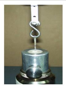
**Fig 2.** Specimen setup for testing the tensile bond strength in a universal testing machine
