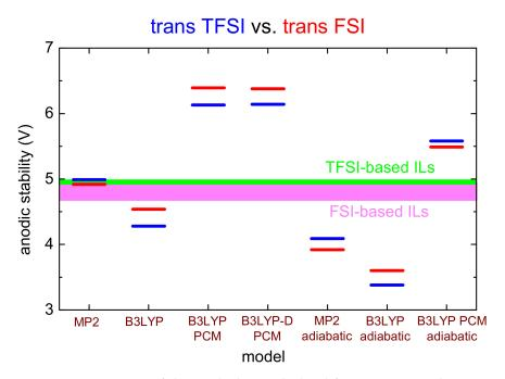
**Figure 2.** Comparison of the anodic limit calculated for trans-TFSI and trans-FSI with various theory levels, in vacuum or in a polarizable medium, considering a vertical or an adiabatic transition between differently charged states. The horizontal colored regions display the interval of values of the experimental anodic stability of the TFSI- and FSI-based ionic liquids investigated computationally in this paper.
