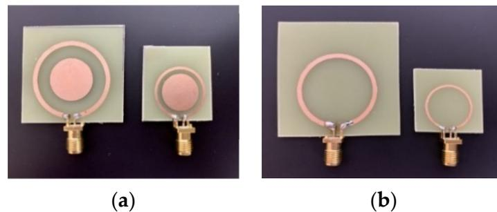
**Figure 3.** Photographs of the (a) tuned resonate couplers with a center pad and (b) single loops without the pad.
