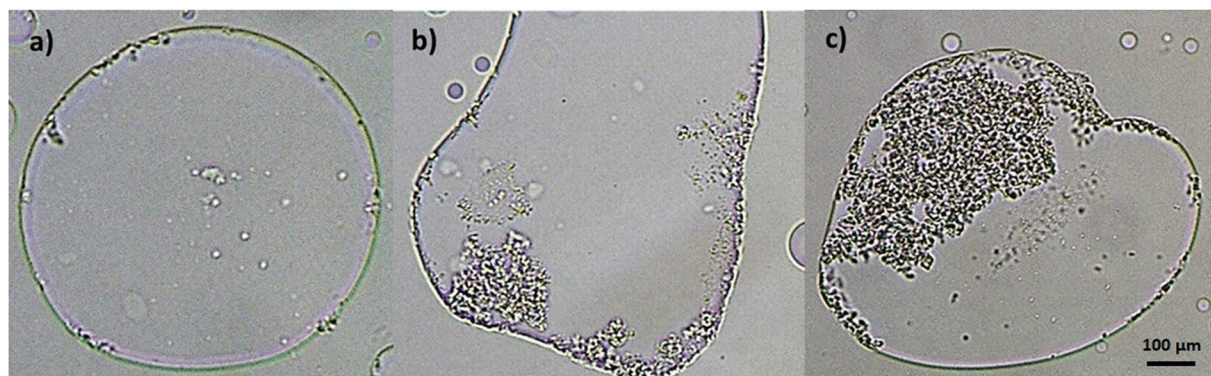
Figure 9. Protein crystals nucleating near the boundary of the droplets (a) and crystals forming within the bulk of the droplets (b,c).
