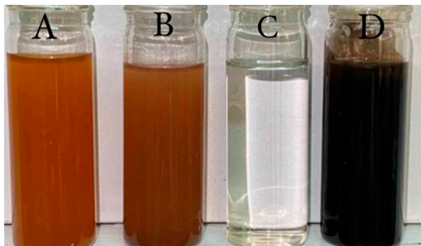
Figure 1. Showing color changing. (A) FeCl 2 and FeCl 3 , (B) change color after stirring, (C) NH 4 OH added to the mixture then change the color to black as show in (D) synthesized Fe 3 O 4 NPs solution.
