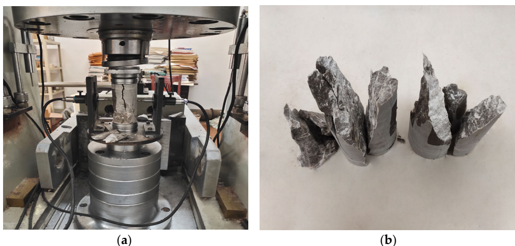
Figure 7. The compressive elastic modulus experiment: (a) test instrument; (b) failure mode.
