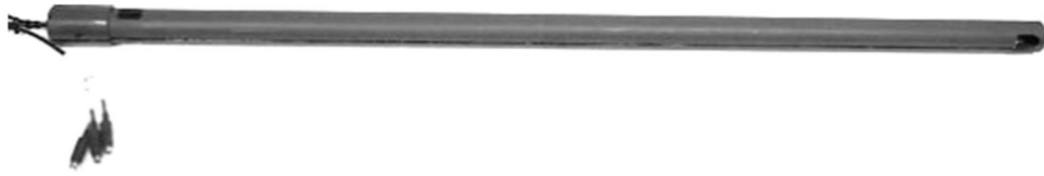
Fig. 8. RTD-instrumented PVC rod for measurement of strata temperatures.
