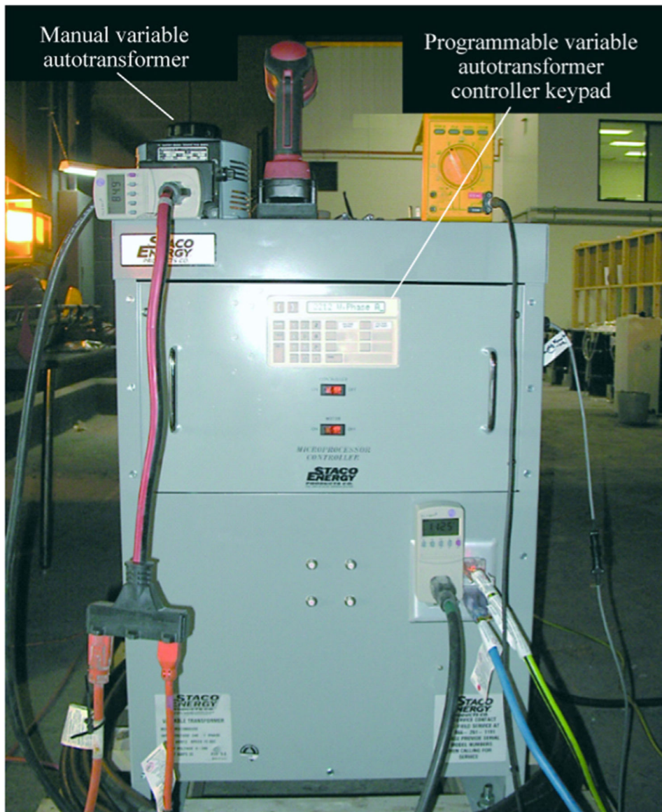
Fig. 5. Programmable variable autotransformer used to control input power (heat) during NIOSH RA heat/humidity testing.
