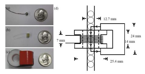
The capability and the repeatability to measure the amplitude and speed of the HNSWs was evaluated by taking 500 measurements at 10 MHz sampling rate for each sensing configuration.
