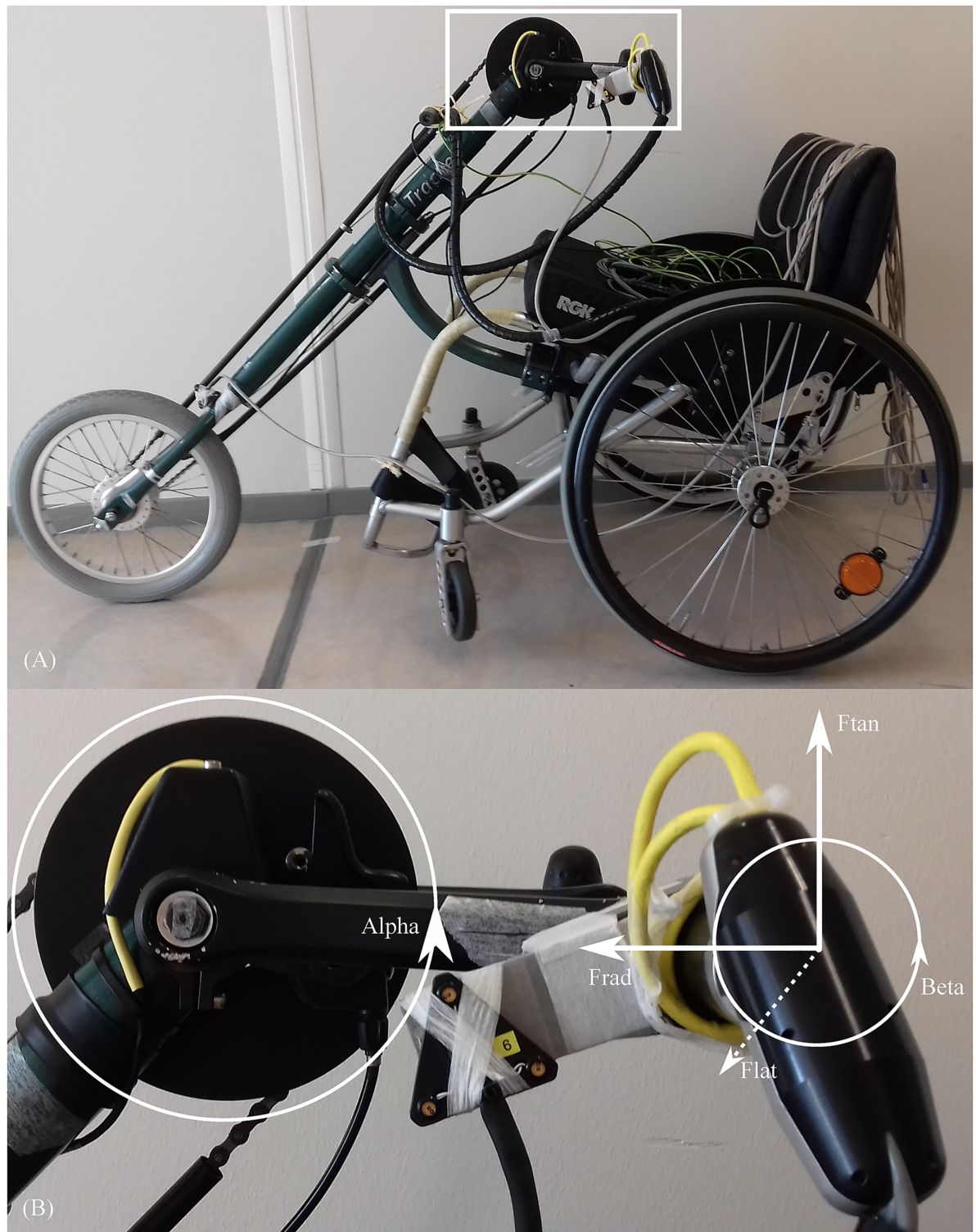
Fig 2. Handcycle and coordinates system. (A) Attach-unit handcycle used in current study with (B) the according 3D coordinates system in the left handlebar. Alpha = angle between crank and axis. Beta = angle between handle and crank. F_{rad} is positive directed towards crank axis, F_{lat} is positive directed leftwards (out of the paper) and F_{tan} is positive directed counterclockwise.
