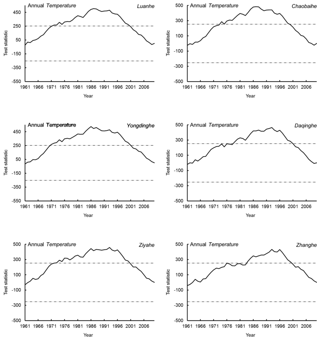
Figure 3. Detection results of the abrupt change point of air temperature in the six sub-basins of the Haihe River Basin.
