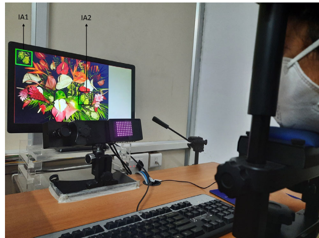
FIGURE 1. Experimental set up, showing the eye tracker and the display monitor. The two Interest Areas (IA) are marked in the search image. The actual experiment was done in a dark room.
