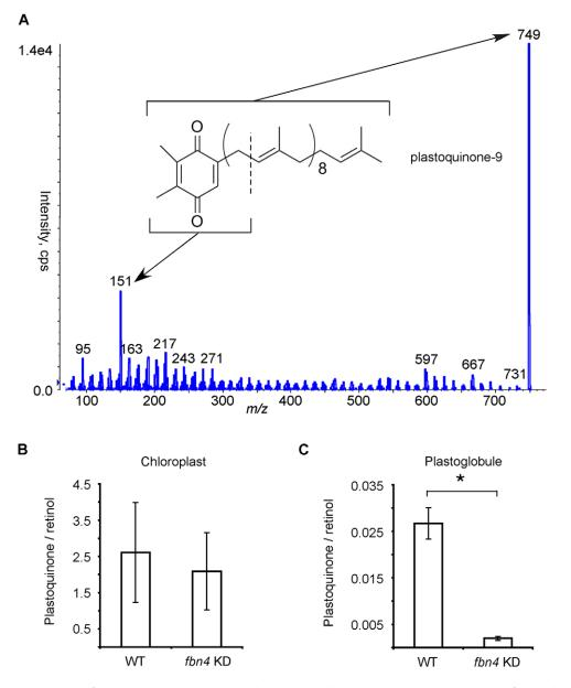
**Figure 3. Analyte at m/z 749.** (A) MS/MS analysis and possible structure. Abundance in WT and *fbn4* KD lipid extracts from chloroplasts (B) and plastoglobules (C), normalized to retinol. Data are means  $\pm$  SD of three measurements; \*, *P*<0.05 using Student's *t* test. Similar results were obtained in two biological replicates for the chloroplasts and three biological replicates for the plastoglobules. doi:10.1371/journal.pone.0047547.g003
