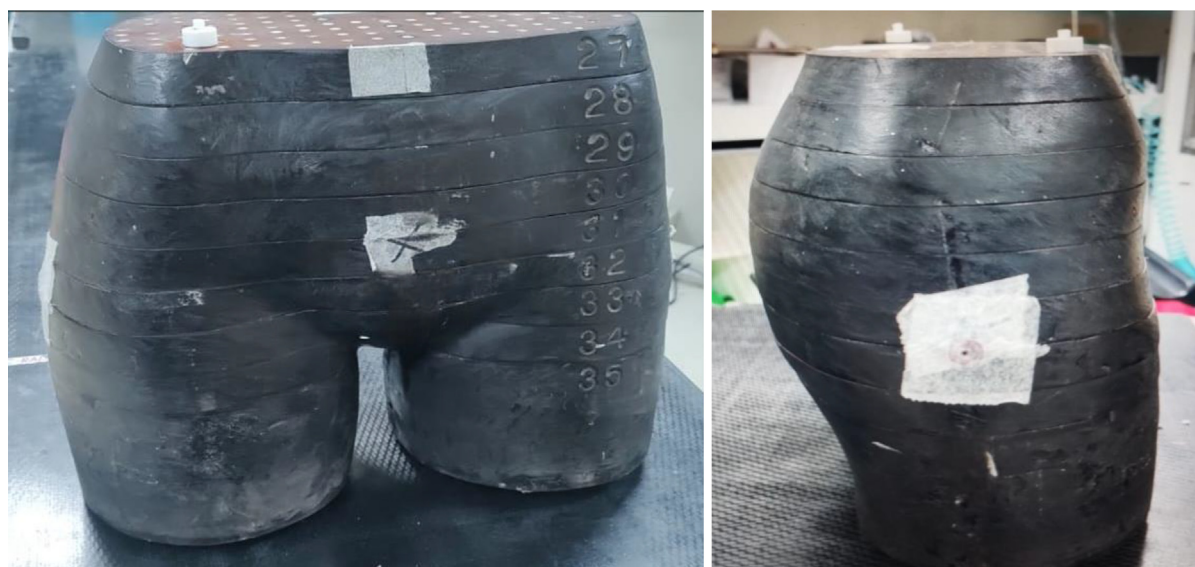
Figure 2 Alderson RANDO female pelvic phantom.
