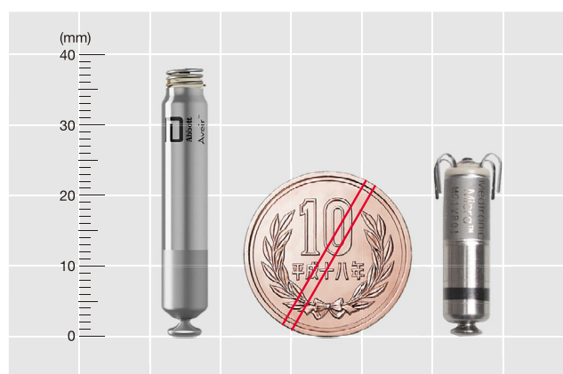
FIGURE 2 Leadless pacemakers available in Japan (as of November 2023). (Left) VVI type, (Right) VVI or VDD type.
