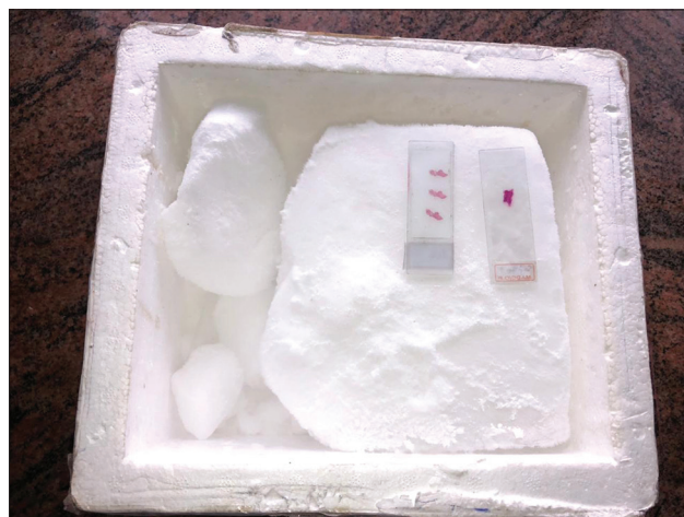
Figure 1: Placement of microscopic slides on dry ice
