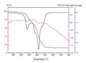
Figure 2. TGA, DTG and DTA curves of MSE-Al.
