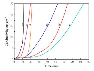
**Figure 6.** Conductivity versus time plots for pure PVC (a); and PVC stabilized by 4 phr of MSE-Al (b); MSE-Al/ZnSt<sub>2</sub> (3:1) (c); MSE-Al/ZnSt<sub>2</sub> (2:2) (d); MSE-Al/ZnSt<sub>2</sub> (1:3) (e); and ZnSt<sub>2</sub> (f).
