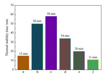
**Figure 5.** Thermal stability time of pure PVC and PVC stabilized by MSE-Al/ZnSt<sub>2</sub> at the content of 4 phr in 180 °C. a, pure PVC; b, 4 phr MSE-Al; c, 3 phr MSE-Al + 1 phr ZnSt<sub>2</sub>; d, 2 phr MSE-Al + 2 phr ZnSt<sub>2</sub>; e, 1 phr MSE-Al + 3 phr ZnSt<sub>2</sub>; and f, 4 phr ZnSt<sub>2</sub>.
