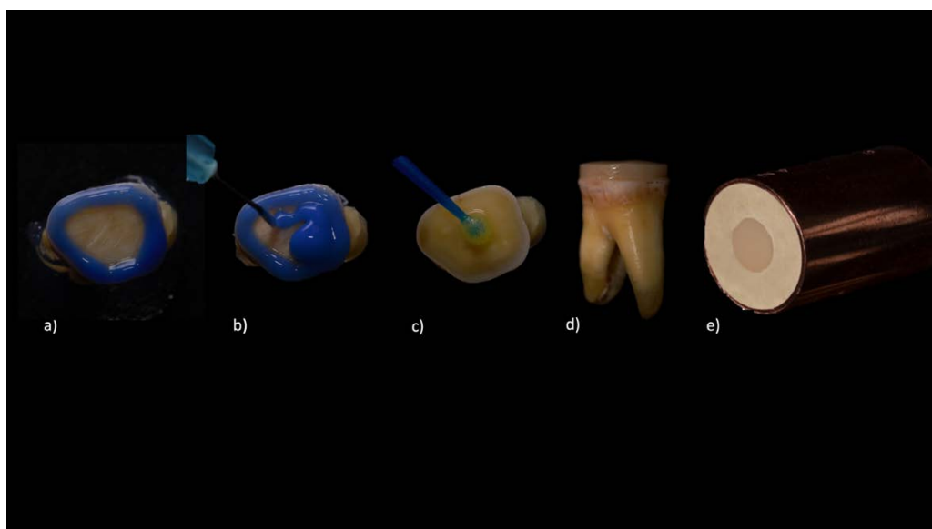
Figure 1. (a) Selective acid etching of peripheral enamel; (b) Dentin acid etching; (c) Adhesive application; (d) Disc cemented onto prepared molar; (e) Insertion in a copper cylinder.
