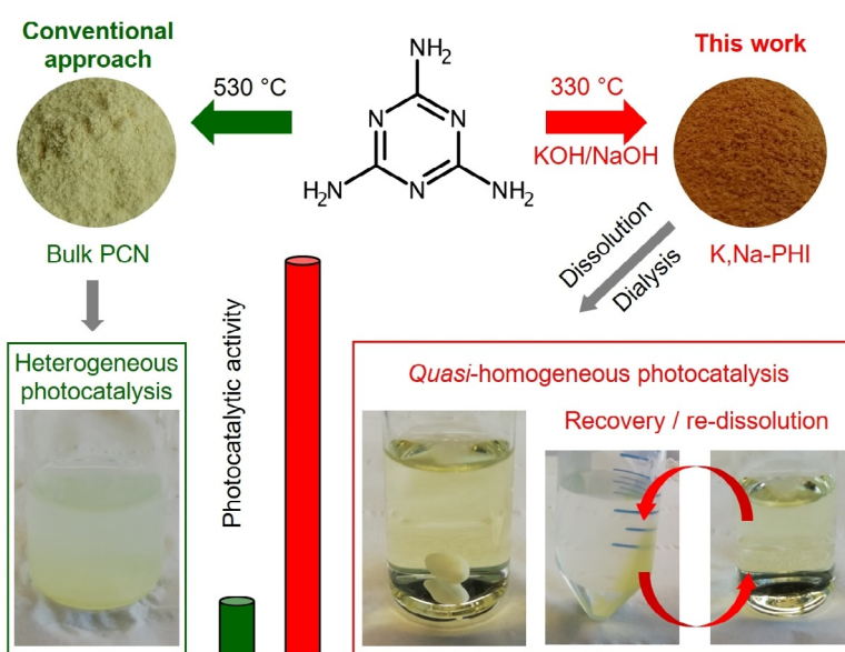
Figure 1. Alkali poly(heptazine imide) is synthesized at comparatively low temperature (330 °C) using a KOH/NaOH melt; after dissolution and dialysis the resulting material is a water-soluble photocatalyst, more active than the bulk PCN, and easily recovered (by increasing the ionic strength via addition of NaCl) and dissolved again, thus enabling recyclability without any loss of activity and selectivity.
