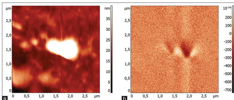
**Figure 3:** Atomic force microscope image of sample topology (a), magnetic force microscopy image of the same sample on the same location (b)
