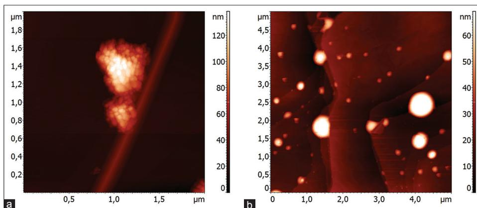
**Figure 2:** Atomic force microscope images of fluidMAG-UC/C magnetic nanoparticles (a) and thin film of dispersion of polyethylene glycol-1000 and phenacetin with 6:1 composition containing magnetic nanoparticles (b) on the surface of highly oriented pyrolytic graphite
