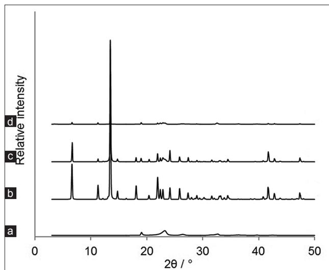
**Figure 4:** X-ray powder diffractograms of polyethylene glycol-1000 (a), phenacetin (b), and their mixtures 1:1 (c) and 6:1 (d)
