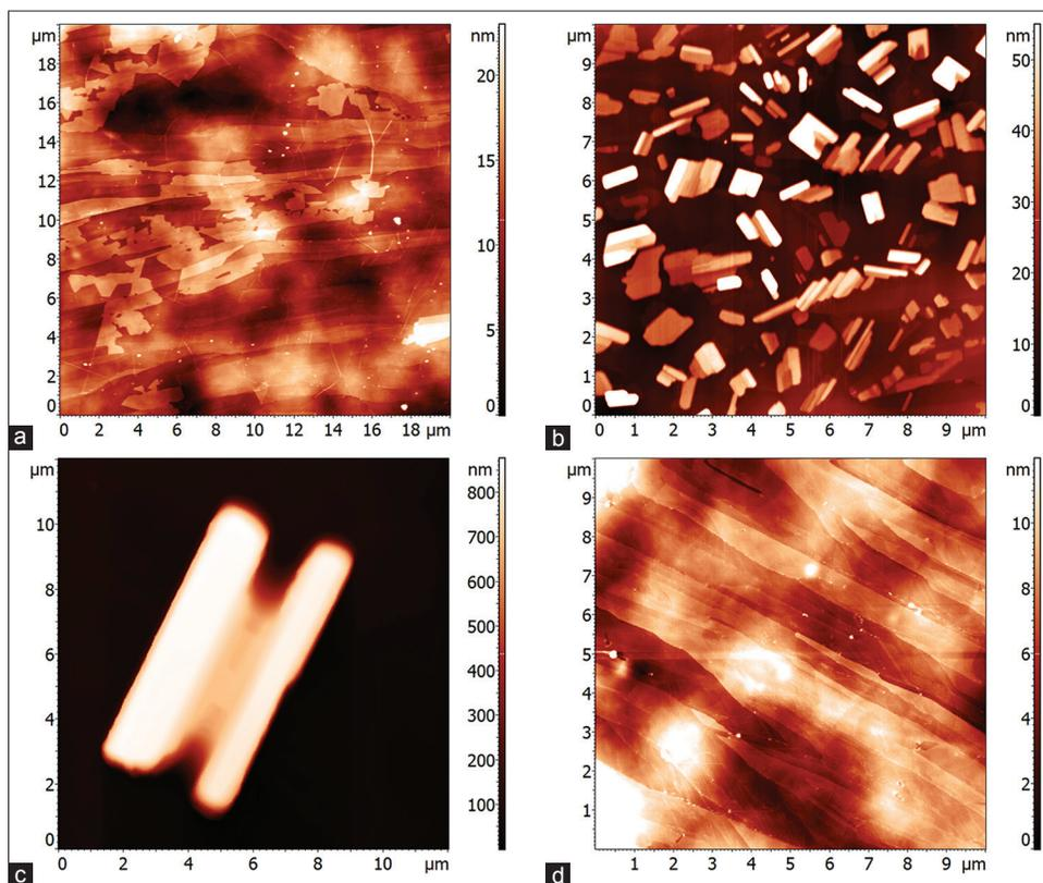
**Figure 1:** Atomic force microscope images of the thin film of polyethylene glycol-1000 (a), phenacetin (b) and polyethylene glycol-1000/phenacetin 1:1 (c) and 6:1 (d) compositions on the surface of highly oriented pyrolytic graphite
