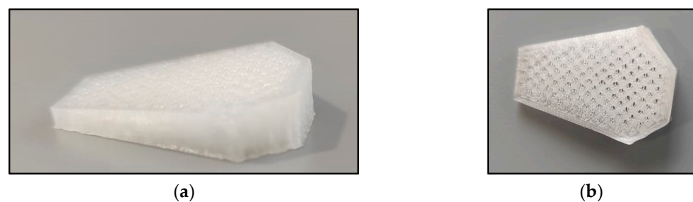
Figure 1. PLA implant. (a) Lateral view of the PLA implant. (b) Frontal view of the PLA implant.
