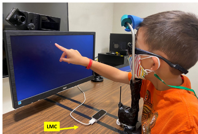
FIGURE 1. Experimental setup. Children held onto a stick placed 5 cm in front of them and, with both eyes open, fixated a cross displayed on a computer monitor at a viewing distance of 35 cm. Once the cross disappeared, a small white dot appeared on the left or right displaced 5 or 10 degrees from fixation. The child was instructed to reach out and touch the dot as quickly and accurately as possible and then return to the stick. The LMC recorded hand movements and was placed 10 cm from the hand's initial starting position.
