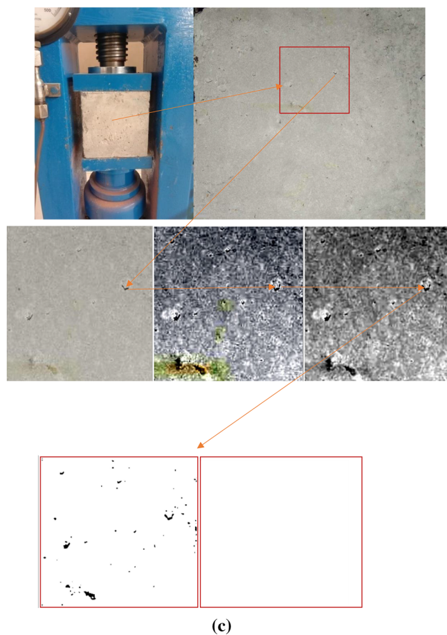
Figure 7. (a) Schematic diagram showing experimental arrangement. (b) Flowchart showing broad steps of spectral clustering algorithm for crack detection. (c) Steps followed by image processing algorithm and removal of noise.
