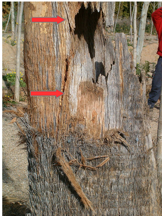
Figure 3. When a decayed desert fan palm stem was statically pulled, collapse was initiated by splitting of the hollow stem. Cracks first appeared above and below the open cavity and initiated at its borders (red arrows) and total collapse only ensued after large longitudinal splitting and delamination.
