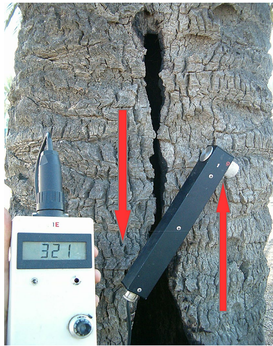
Figure 1. The strain gauge sensor was placed obliquely over an open cavity in a date palm, recording high shear deformations. The red arrows show the direction of the strain, producing shear as the two halves of the stem seemed to slide over each other, while a static pull was being applied.
