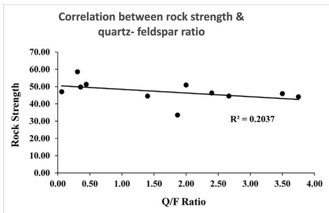
Figure 8. Correlation between rock strength and quartz-feldspar ratio.
