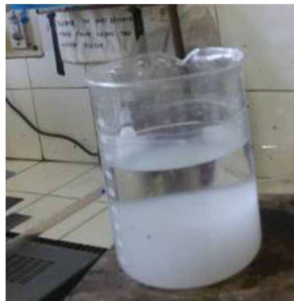
Fig. 2 Three layers formed in the beaker after the electrocoagulation process
