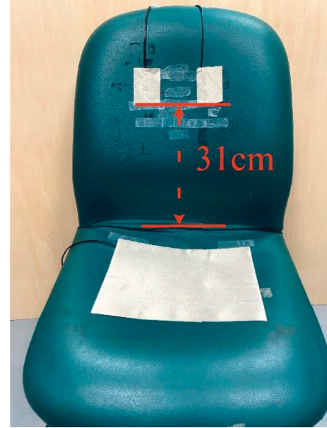
FIGURE 2: Photograph of conductive textile configuration.
