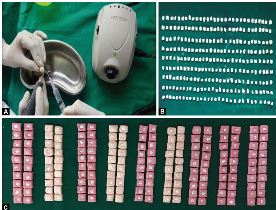
Figs 2A to C: Enamel slabs including at least 1 mm of underlying dentin were sawn from the teeth using a diamond disk under water irrigation. The slabs were embedded in acrylic resin
