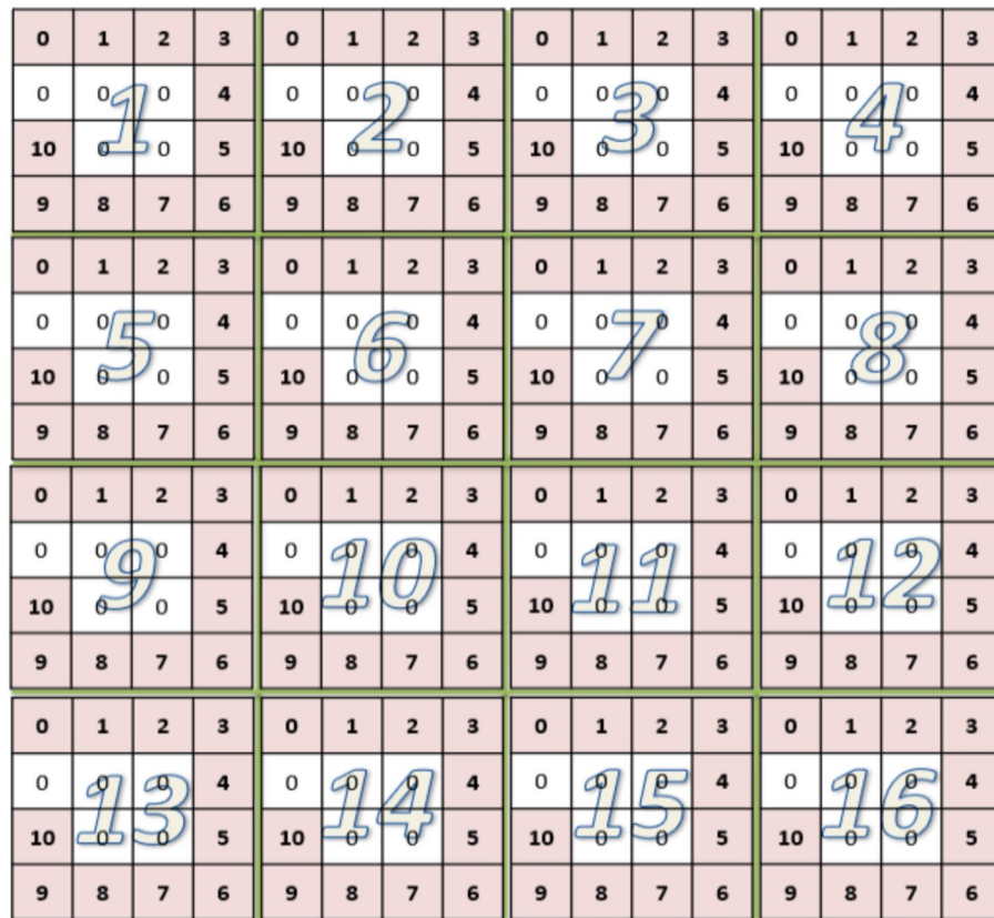
Figure 6. 16 4*4 data grids arranged sequentially one after another to form a Mosaic data structure as the network input to keep the time feature of the original data.
