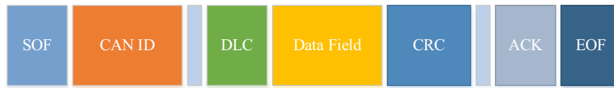
Figure 4. CAN data frame structure, where SOF represents Start of Frame, DLC represents Data Length Code, CRC represents Cyclic Redundancy Check, ACK represents Acknowledgement, and EOF represents End of Frame.
