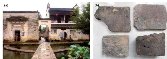
Fig. 1 (a) Hongcun village of Anhui province; (b) the brick samples were from a historic house in Hongcun village, Anhui province, there was no difference between the four bricks, the water content of four bricks was 13 wt%.
